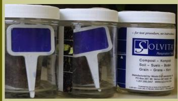
Some biological soil tests use color-changing paddles to indicate soil respiration, which serves as a proxy for soil nitrogen.
